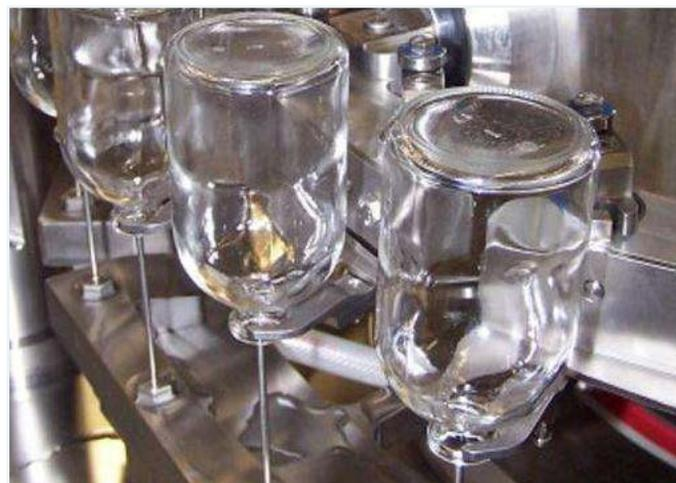
**Figure 1** Washing needles penetrating vials
